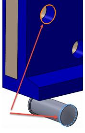
If the **Lock rotation** box is ticked as shown the rivet is locked and will not rotate.
