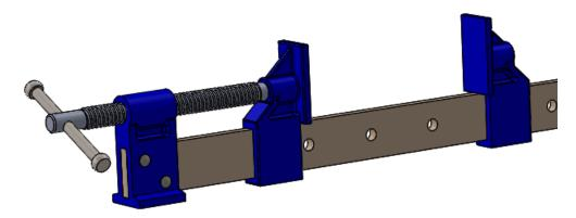
To enable the slider 2 to react as it would in reality additional mates can be added.
