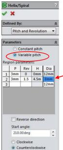
Then without exiting the command, select **Variable pitch** and as in the other side change the diameter to **8mm** keeping the revolution at **1.5.**
