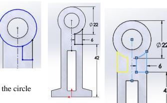
Mirror about the centreline and **Extrude Cut** using **Mid Plane** by **25mm**.
