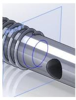
On the face of the triangle draw a new sketch. Use **Convert entities** to transfer the triangle onto this new plane.
